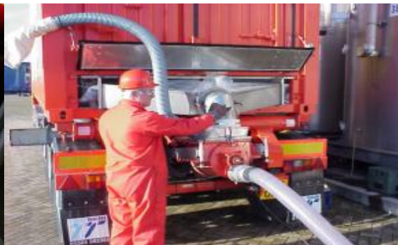
Rotary valve set up for "discharge Operations".
