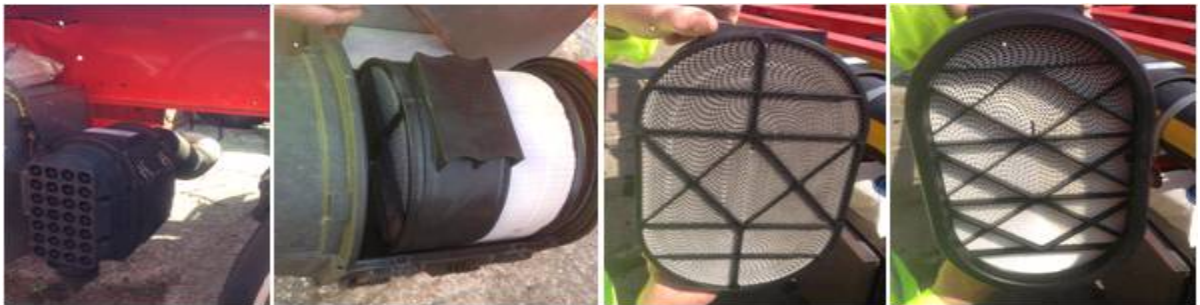
Air intake filtration system for SDU chassis.
