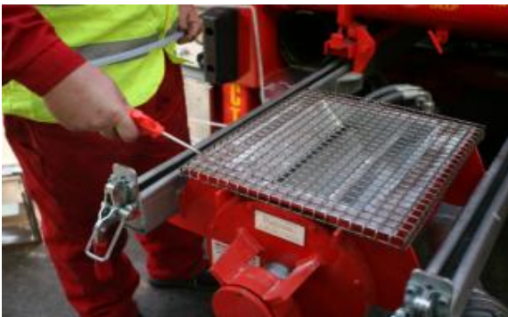
Rotary Valve Cleaning with safety grid in place.
