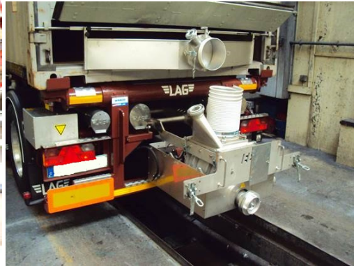
Sliding out the rotary valve for set up of equipment
