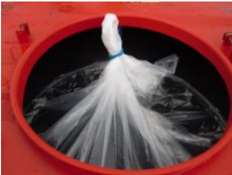
Swan neck correctly fitted and tied
