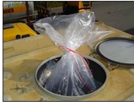
Swan neck incorrectly fitted and tied
