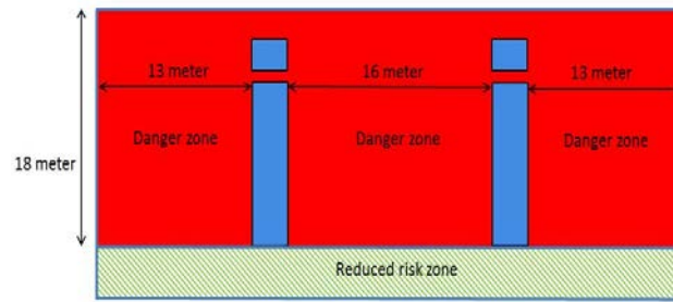
Both silo trailers in tipped position with an overlapping danger zone
