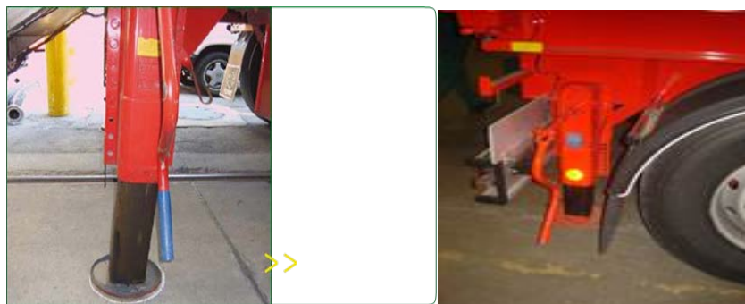
Bent stabilizing legs and should be changed
