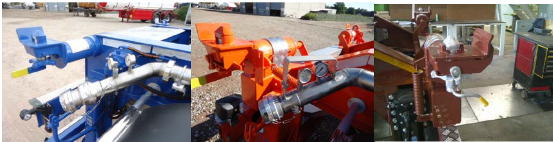
Twist locks with indicators and heel plates
