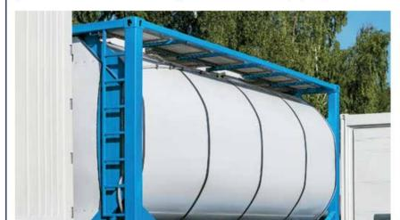
are made in Germany, w capacities ranging from 12,000 litres to 24,000 litres. The tanks are fitted into 20-foot box containers in accordance with precise specifications.
